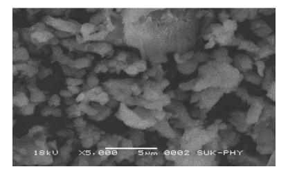
Figure 6. SEM image of Calcinated egg shell
