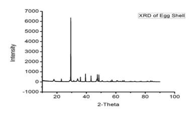
**Figure 4**. XRD spectra of egg nanoparticles
