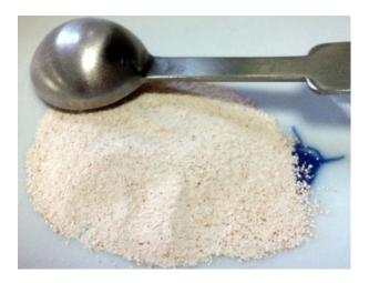
Figure 1. Calcined egg shell powder
