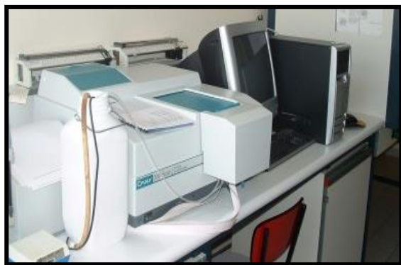
Figure 2 UV spectral analysis setup
