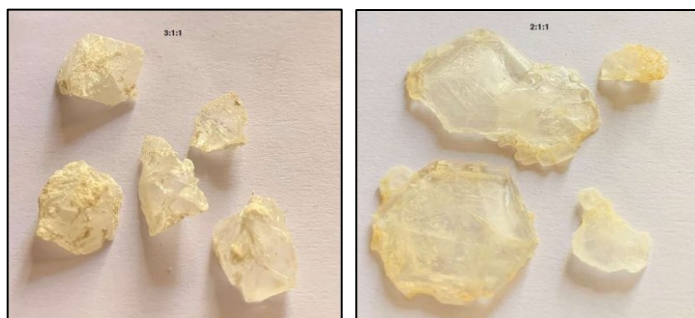
Figure 2 a & b the grown hybrid crystals of KDP:ADP: L-Arginine in the ratio of a) 2:1:1 and b) 3:1:1
